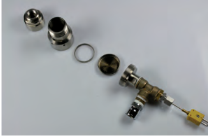
Figure 1: Filter holder for planar filters and filter sleeves by the Paul Gothe company; Image: TFZ
