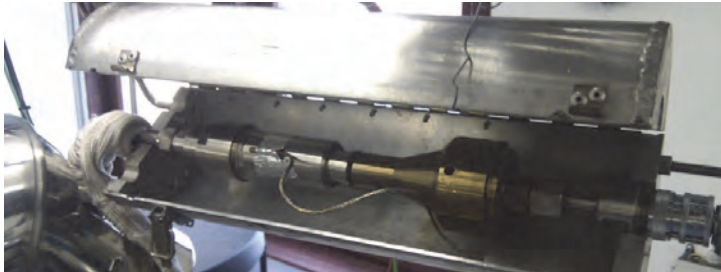
Figure 3: Filter sleeve holder and planar filter holder in the heating case (with temperature measurement); Image: ZAE Bayern
