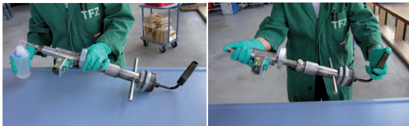
Figure 3: Rinsing of the sampling probe with distilled water and acetone; to the left: filling the liquid into the probe; to the right: distributing the liquid throughout the probe by shaking while sealing both openings off; Image: TFZ
