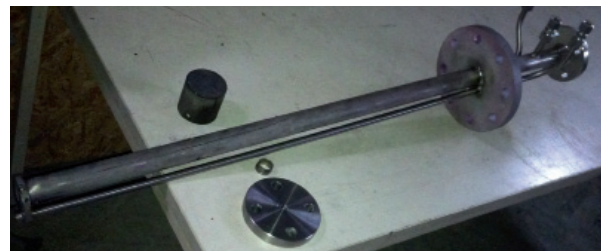
Figure 4: In-situ filter with integrated catalyst.
