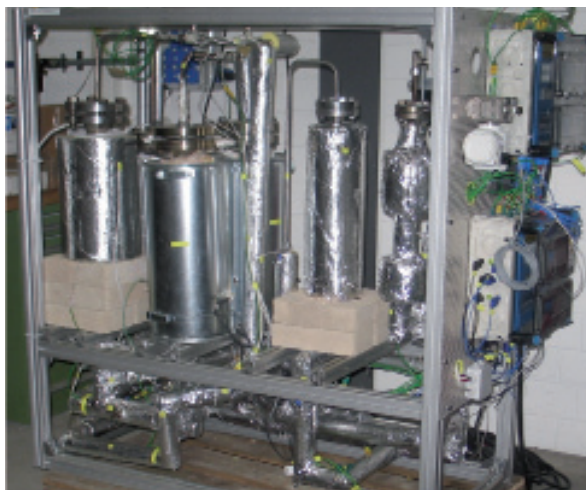
Figure 3: Laboratory system for gas cleaning and methanation.
