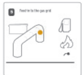
5 The upgraded gas is dried and compressed and is injected as biomethane into the natural gas grid.
