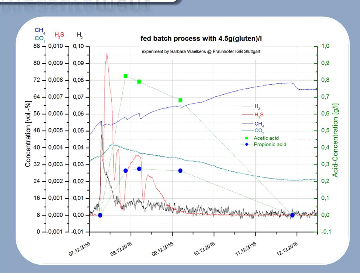
An old prototype was used to detect the gas concentrations of a test fermenter at the Fraunhofer IGB in Stuttgart.
