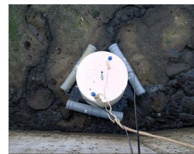
Fig. 2: Closed chamber measurement of methane emission rate at the surface of an open digestate storage tank (© Torsten Reinelt, DBFZ).
