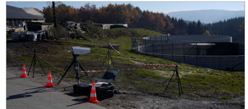
Fig. 1: TDLAS measurement setup for the determination of the emission rate from an open digestate storage tank (© Carsten Tilch, DBFZ).
