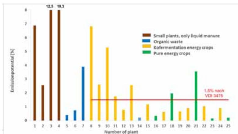
Figure 1: Emission potential of 25 biogas plants, analyzed at a digestion temperature of 20°C with different digester design and different substrates.
