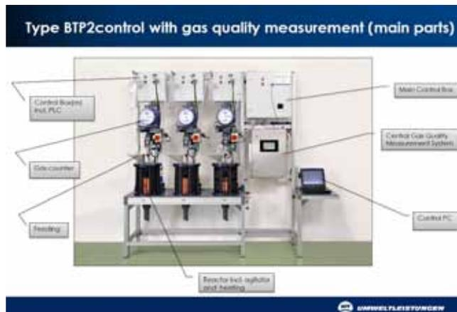
Figure 1: BTP 2 CONTROL incl. central gas analysis module
