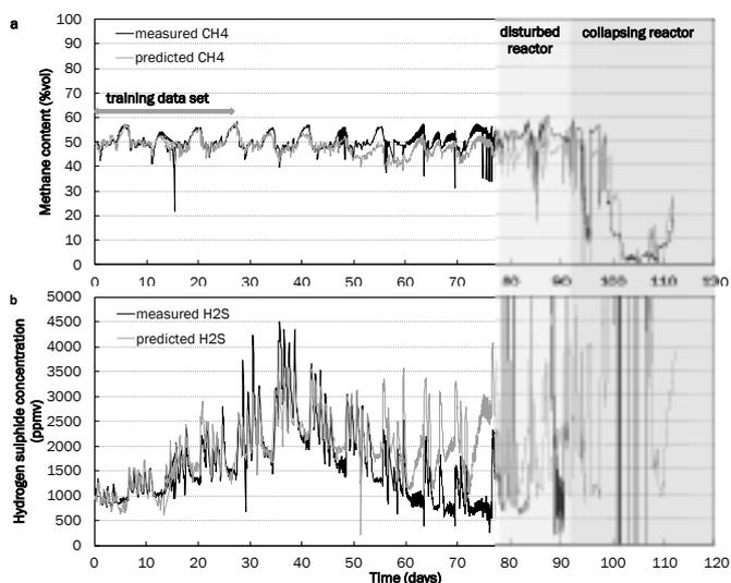
Figures 2a and b. Time series of measured and e-nose predicted concentrations of a) methane and b) hydrogen sulphide.
