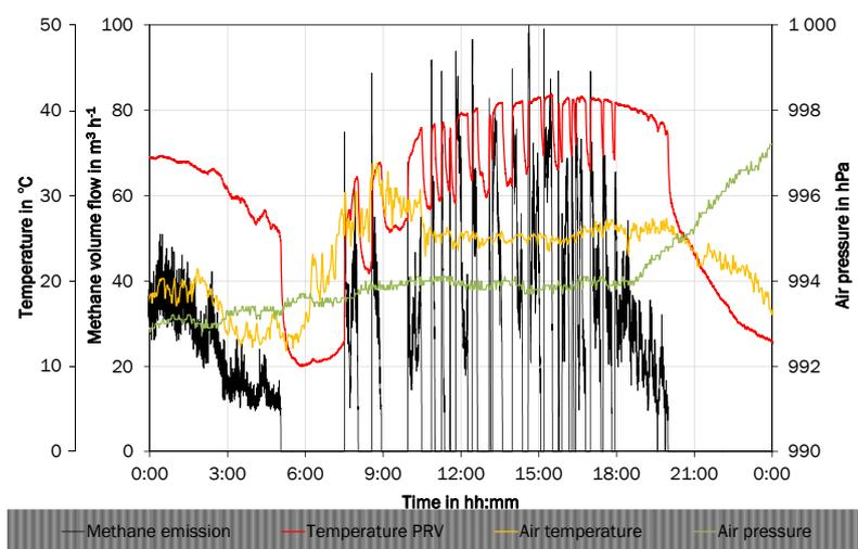
Figure 2: Diurnal variations of an investigated PRV and the atmospheric conditions (modified from Westerkamp et al., 2014)
