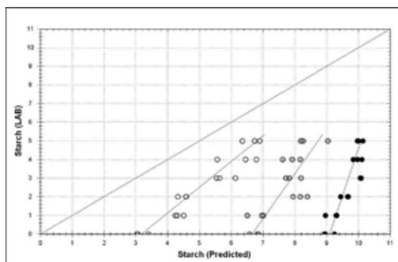
Figure 1: Regression lines of predicted starch contents in slurries with different dry matter (DM) contents. Calibrations were performed in water; shown values are predictions, based on the calibration of starch in water. Colour and corresponding DM (in %) from left to right: white (0.38), grey (0.94), black (1.5). The angle bisector represents the calibration with 0 % DM (data points not shown).
