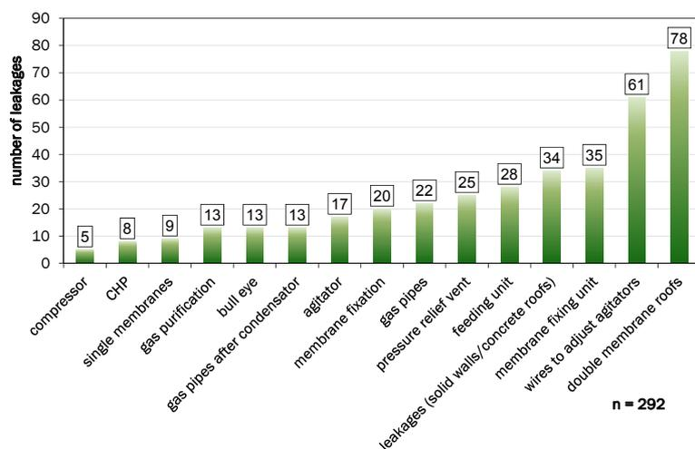
Figure 1: Number and location of detected leakages (modified from Clemens, 2014)
