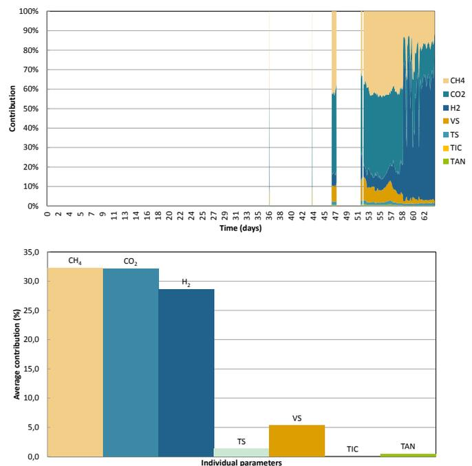
Figure 2: Contribution of the individual parameters in the computation of  $T^2$  values exceeding upper control limit for the selected overfed reactor. a. According to measurement date; b. Averaged contribution for a typical out-of control situation.
