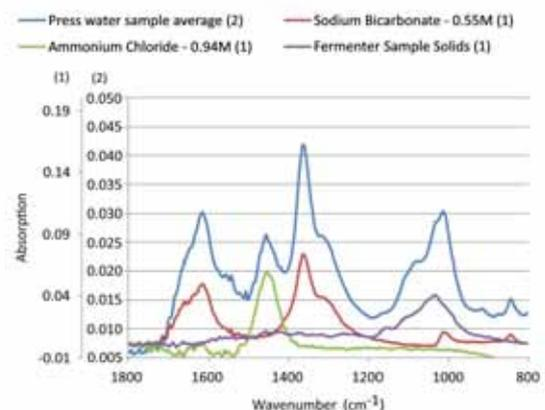
Figure 1: MIR spectrum of AD sludge and press water in comparison to spectral data from ammonium and sodium bicarbonate.
