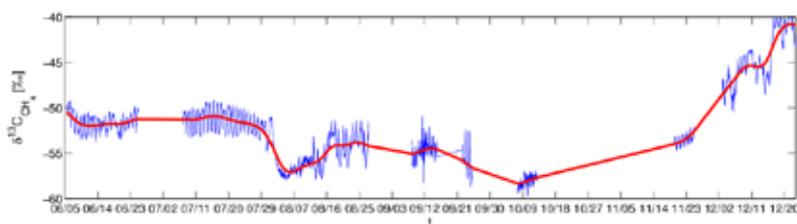
Figure 1: Monitoring of  $\delta^{13}\text{C}_{\text{CH}_4}$  at a pilot-scale maize-digester with  $190\text{m}^3$  at DBFZ
