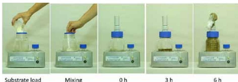
Figure 1: Foaming test by use of LEIPZIG F0AM TESTER (experimental set-up: 10 g protein powder in 490 g active digestate, 37 °C)
