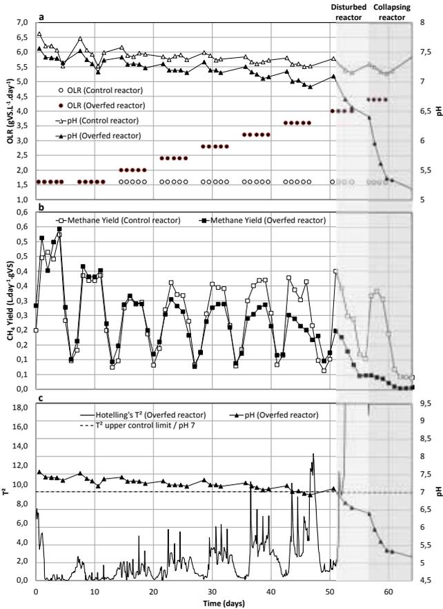
Figures 1a, b and c: Time series of reactor state monitoring for the control reactor and 1 overfed reactor. a. OLR and pH; b. Methane yield; c. Relationship between T<sup>2</sup> and pH for the selected overfed reactor.
