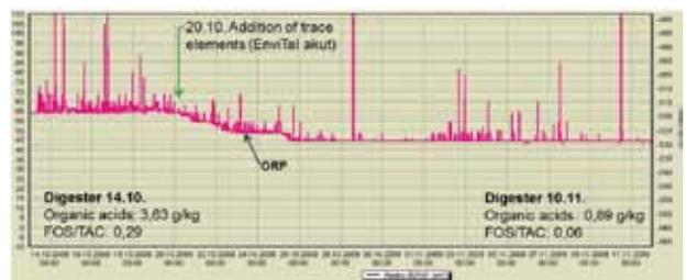
Figure 3: Redox measurement at a biogas plant with trace element deficiencies
