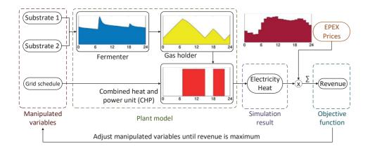
Figure 1 Scheme of model-based process optimization
