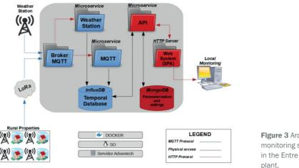
Figure 3 Arquitecture of monitoring system used in the Entre Rios do Oeste
