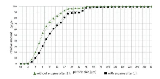
$\label{eq:Example: Figure 1} \mbox{Particle size distribution measured with laserlight backreflection in culture broth with and without enzyme addition$
