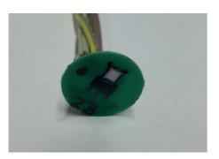
Figure 2 Interdigital electrode on a printed circuit board
