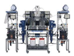
Fig. 3 Biogas Test Plant BTP2-control with automated feeding system
