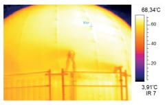
Figure 1 (right) Temperature effects on the available gas storage capacity; (left) surface temperatures of up to approx. 68 °C on the outer side of the light gray protective membrane of the DBFZ research biogas plant / Picture by IR- camera (Mauky/DBFZ).
