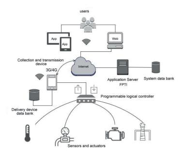
Figure 2 Details of the developed arquitecture for the monitoring system.
