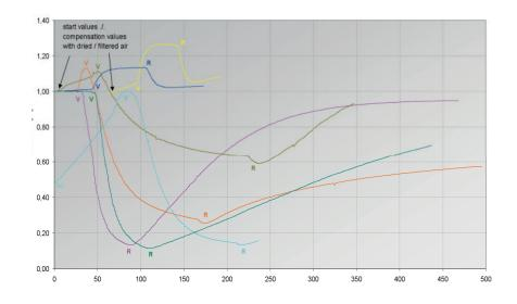
**Figure 1** Representative sensor characteristics related to constant start values – the time intervals are divided into a phase of reoxidation (R) and a phase of VFA flow (V) with 100 ppm analytical pure acetic acid; 5 sensors exhibit amplitudes between -60 % and -89 %, 2 sensors +12 % and +22 %; the time constants between ~6.3 s and ~38 s yield spectra with high accuracy; in the laboratory calibration carbonate buffer solutions are adjusted with pH measurement
