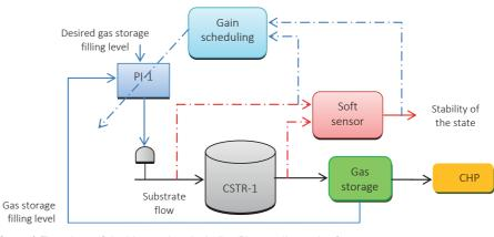
Figure 1 Flow chart of the biogas plant including PI controller and soft sensor
