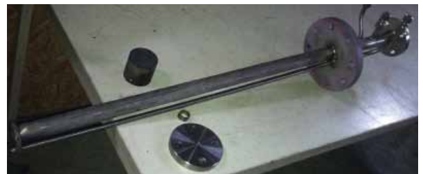
Figure 4: In-situ filter with integrated catalyst.
