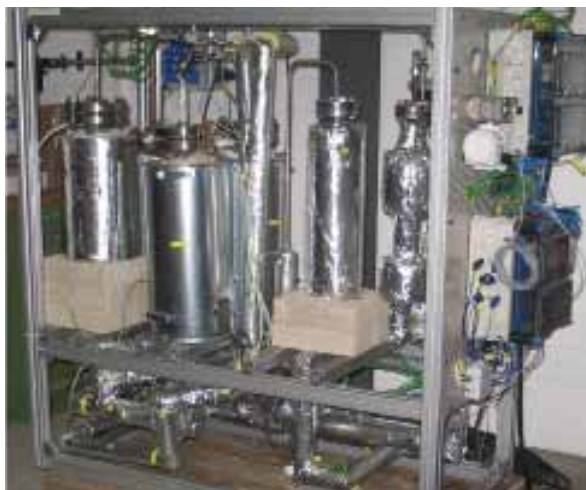
Figure 3: Laboratory system for gas cleaning and methanation.
