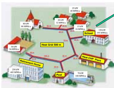
Fig. 3: Integration of a woodgas CHP (45 kW<sub>el</sub> // 90 kW<sub>th</sub>) in a DH project
