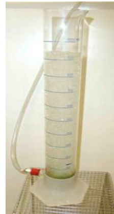
Figure 6.3-2: Foam generator with model foam (Source: UFZ)
