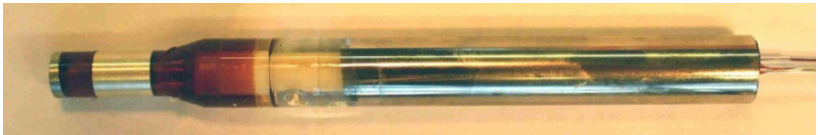
Figure 10.1-1: Amperometric hydrogen sensor (Source: KSI)
