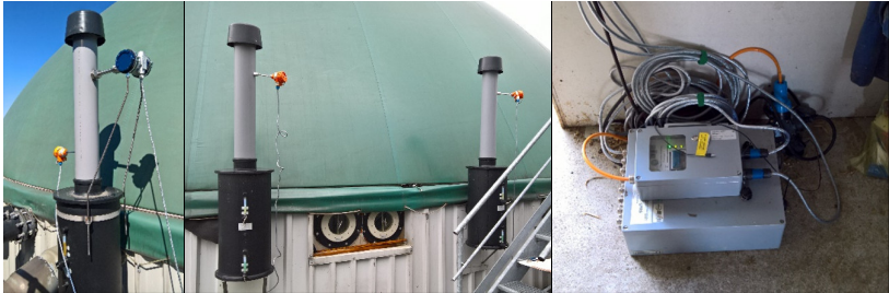
Figure 5.7-3: Exemplary measurement setup at the PRVs of an agricultural biogas plant; Left: Flow velocity and temperature sensor installed at the PRV of the main digester (cp. Fig. 5.7-1); Centre: Temperature sensors installed at PRVs of the gastight covered digestate storage; Right: Data logger; Figure modified from (LIEBETRAU et al. 2017)
