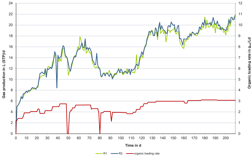
Figure 7.4-4: Gas production and organic loading rate of two continuous fermentation tests in parallel test (Source: DBFZ)
