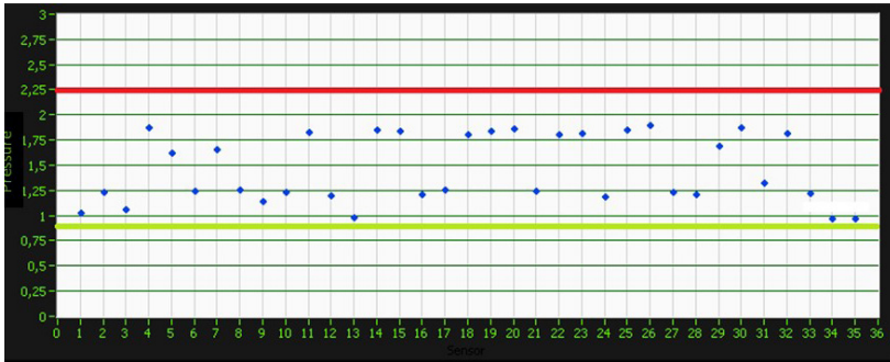
Figure 8.8-2: Part of the screenshot to record the existing pressures at the individual measuring points. Green \triangleq Ambient pressure, red \triangleq Perm. Max. Pressure. Blue corresponds to the prevailing pressure at each measuring point
