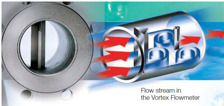
Figure 5.1-1: Principle of vortex method (Source: ABB)
