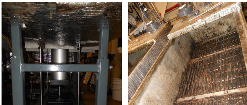
Figure 8.7-3: Pneumatic piston beneath dry digester and grating pulled down onto material to simulate pressure from material height inside the bunker (Source: InnoTech)
