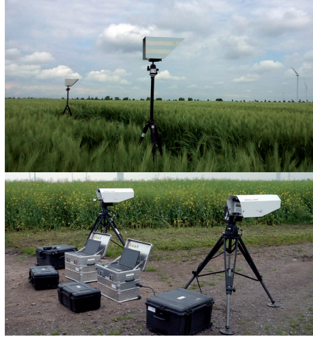
Figure 5.6-1b: To the left: reflector modules, to the right: laser spectrometer (Source: DBFZ)
